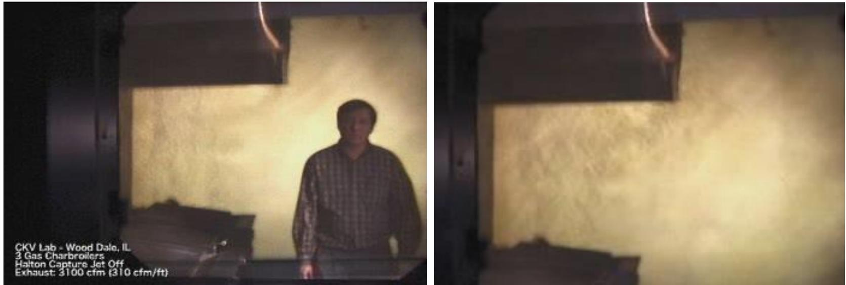
The draft generated by the man's walk is enough to spread the thermal plume. **Imagine what would be the effect of diffusers** wrongly designed or bad balanced between the cooking area and the rest of the kitchen.
